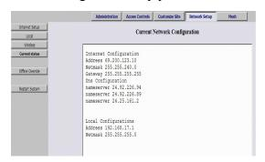
If you have access to Checkbox through a wireless client you can find this address in the Checkbox Administration Screen by clicking on Network Setup in the top menu and Current Status on the left hand menu. On the second line you will see a listing for "Address". This is the IP address assigned by your Internet Service Provider (ISP), or your internal router, to our system.
